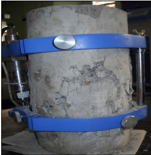
Fig. 3:- SFRC cylinder at failure
