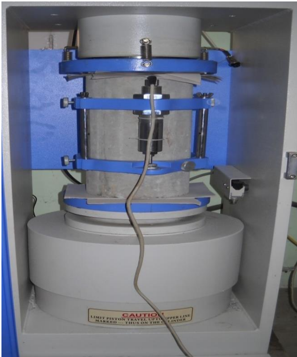
Fig. 2:- Specimen with Compressometer in ACTM
