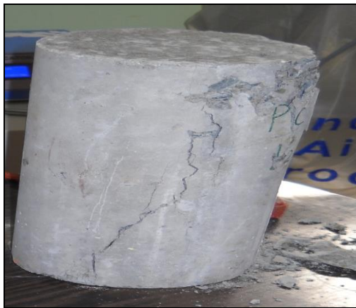
Fig.4:- Plain concrete cylinder at failure
