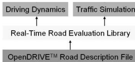
Figure 1. Typical incorporation of an OpenDRIVE® file into a simulation application
