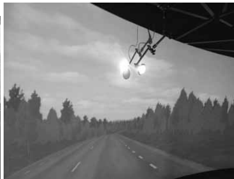
Figure 3. The lamp with shadow and reflection on the screen. Photo: VTI
