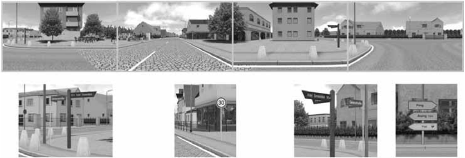
Figure 3. Representation of the crossing used to judge on spatial resolution. The upper image is composed of four images in the direction of 0°/90°/180°/270°. The lower part shows details that were used to decide on readability
