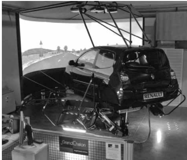
Figure 1. SAAM dynamic driving simulator (Arts et Métiers ParisTech / Renault)
