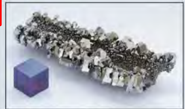
High-purity niobium crystals, electrolytic made, as well as a high-purity 1 cubic centimeter anodized niobium cube for comparison (photograph from Wikipedia).
