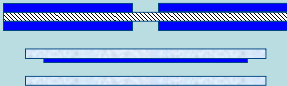
Dual section (series) Design - double metalized, single layer dielectric
