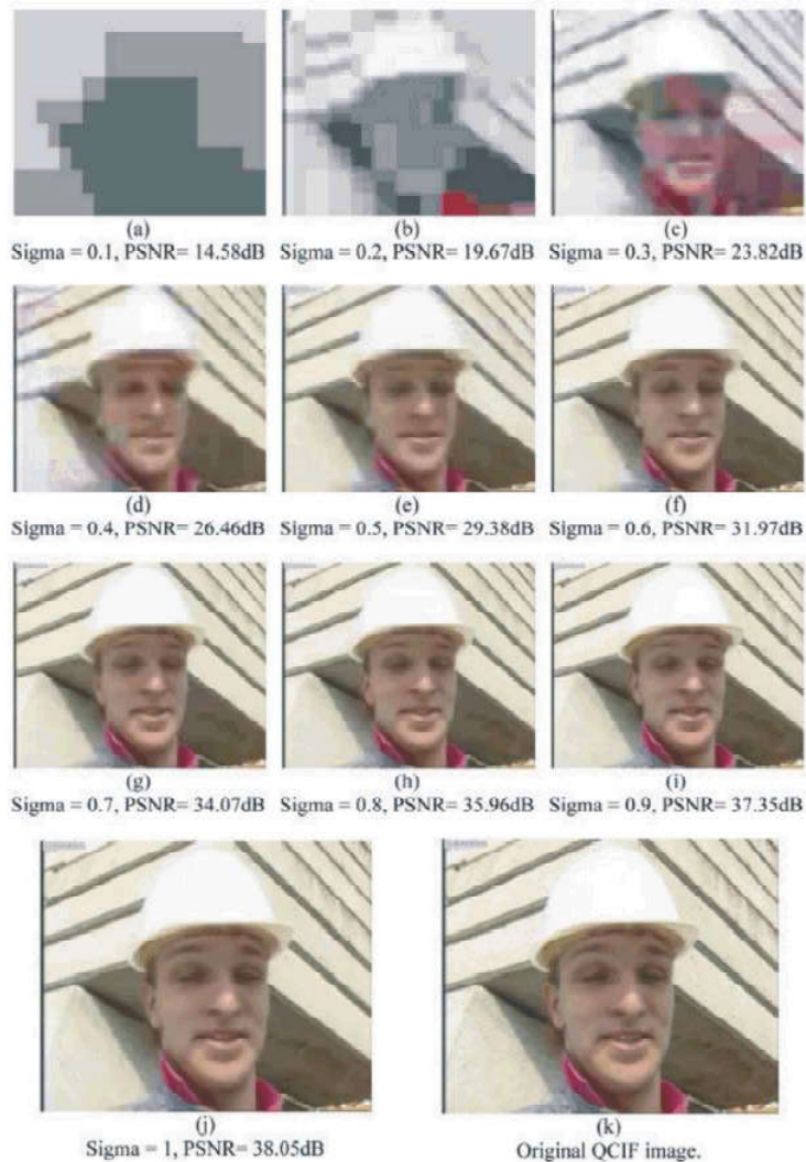
Fig. 5: The 1st frames of the QCIF Foreman sequence reconstructed by the central decoder corresponding to sigma = 0.1 to 1
