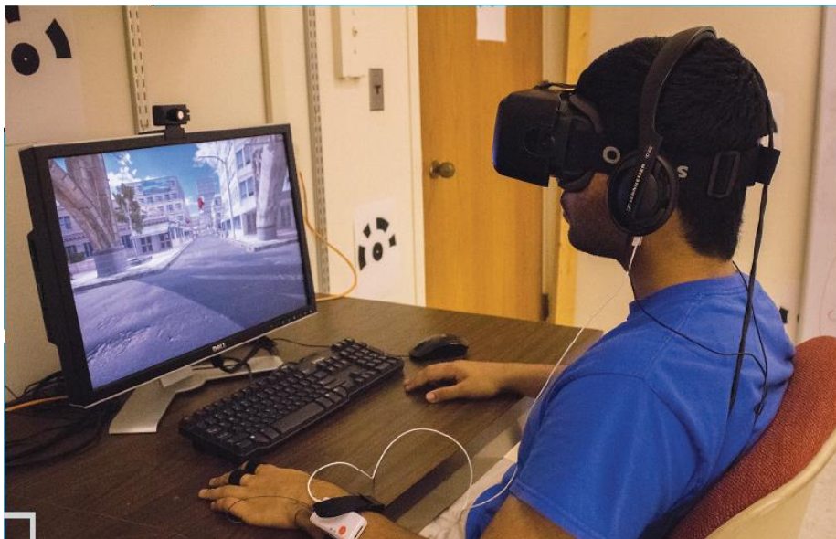
Figure 4 – VR simulation of UAV flight during biometric data acquisition
