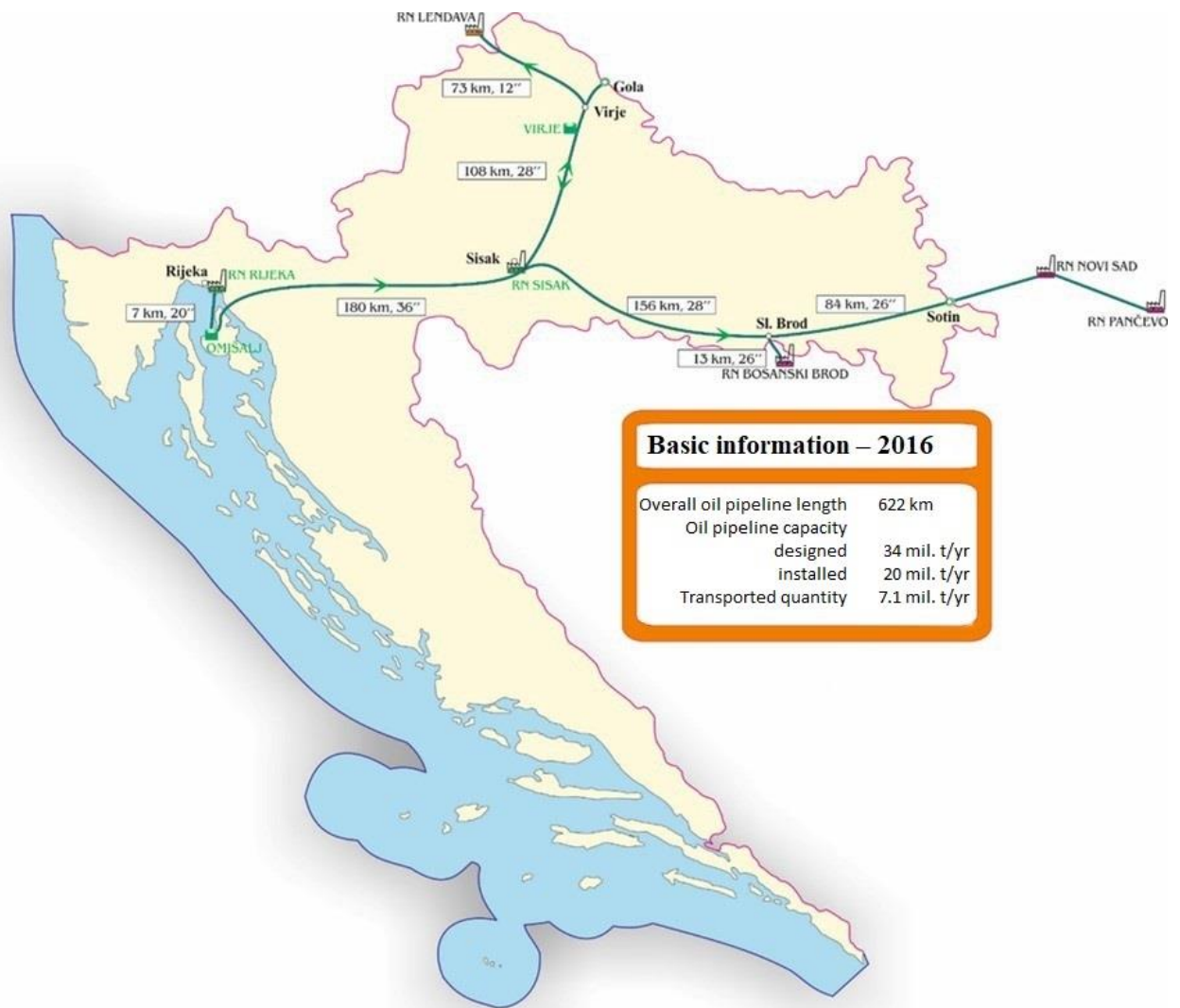
Figure 6.2.1. JANA F d.d. oil pipeline system
