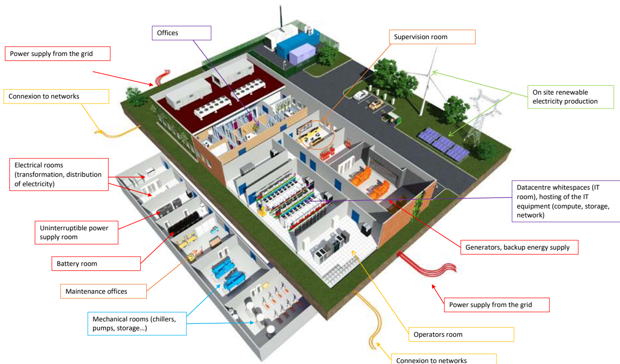
Figure 9 - Representation of a standalone data center and its different spaces (technical and IT spaces)
