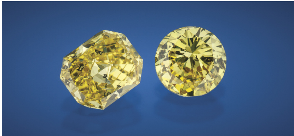
Figure 8. These two bright yellow diamonds (1.03 and 1.02 ct) are from alluvial deposits in the Zimmi mining area in southern Sierra Leone. In the rectangular stone, several black graphitized feather inclusions are visible. Photo by Robert Weldon.
