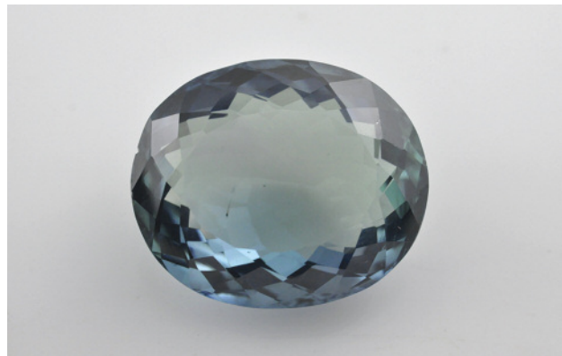
Figure 5. This 40.50 ct greenish blue specimen was identified as irradiated spodumene. Photo by Gagan Choudhary.
