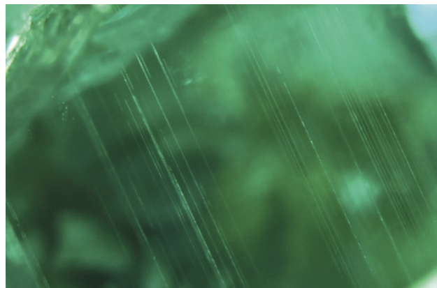
Figure 5. Growth tubes parallel to the prism faces of the crystal are visible in this Musakashi emerald. Photomicrograph by S. Saeseaw, brightfield illumination. Image width 27 mm.
