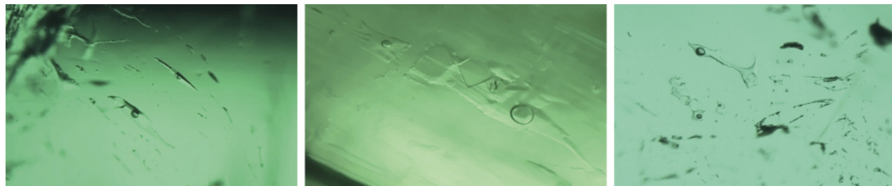
Figure 20. Left: In Colombian emeralds such as this one from Muzo, liquid was often associated with a gas bubble as well as a large colorless cubic crystal. In this sample, some smaller colorless and dark crystals are also visible. Center: Elongated blade-like multiphase inclusions hosting a gas bubble and a large colorless cubic crystal (slightly larger than the bubble) in an emerald from Coscuez. Right: In some cases, the multiphase inclusions were not jagged or elongated blades but irregularly shaped. Here the multiphase inclusions from a Coscuez emerald host a gas bubble, a large colorless cubic crystal (about the same size as the bubble), and some smaller crystals. Photomicrographs by S. Saeseaw, brightfield illumination. Image widths 13 mm (left) and 8 mm (center and right).
