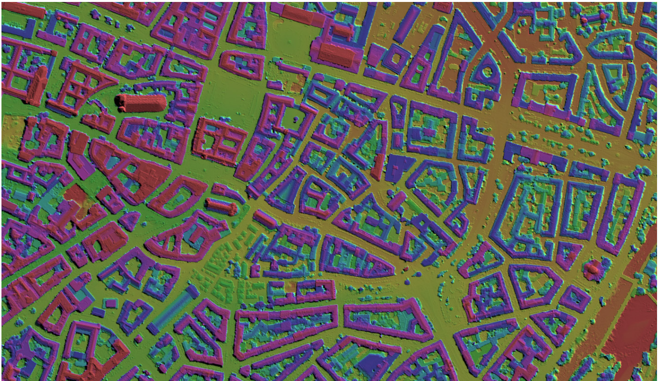
Figure 2 Terrain-shaded relief (TSR) image of DSM generated by NGATE after the triangulation of images.
