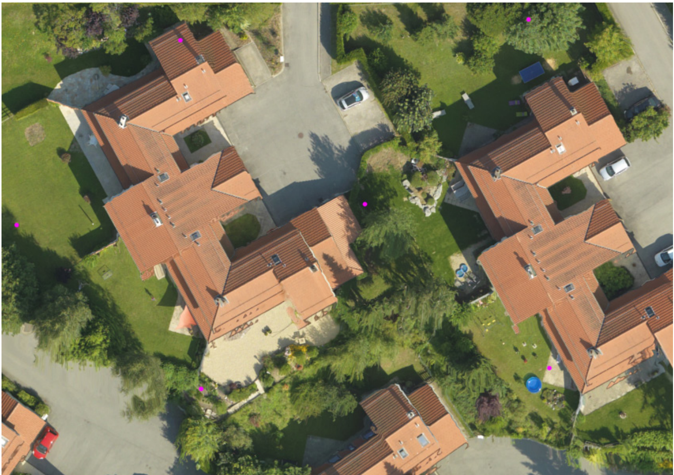
Figure 18 Manually measured ground points, 124 (red dots) and an orthorectified image generated from the DSM and UAV images.
