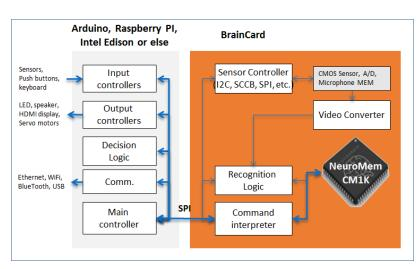
The RECO\_EN and VI\_EN lines must also be pulled up in order for the recognition stage to run and bit 0 of the RSR register must be set to 1. Beyond this setup, the controller simply samples the DATA bus of the CM1K upon the rise of its CAT\_VALID pulse and formats or pushes it As IS to the USB controller for output.
