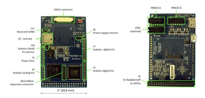
NOTE: The J9 connector and the 2 PMOD connectors are no longer mounted on the new version of the BrainCard.
