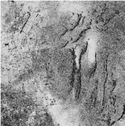
Figure 5a: Correlation over Las Vegas ERS Tandem data, 5 looks, 20 meter azimuth spacing. Correlation displayed from 0.0 to 1.0 as intensity.
