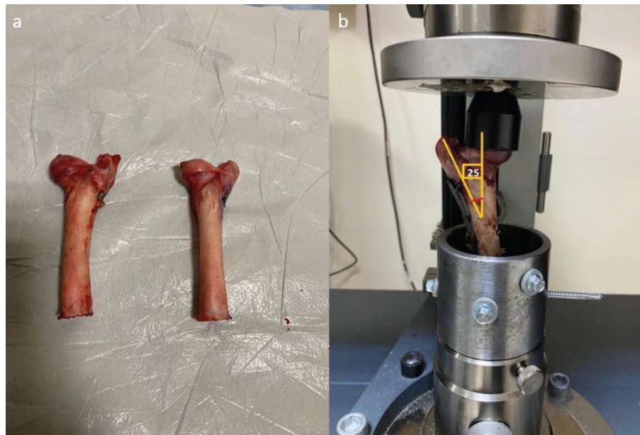
Figure 6. A, Femur model. B, Axial compression tests for femur model.
