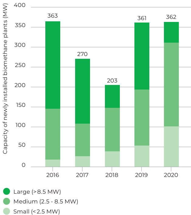
Figure 3 Size of newly installed biomethane plants in MW (EBA, FNR) 6, 7
