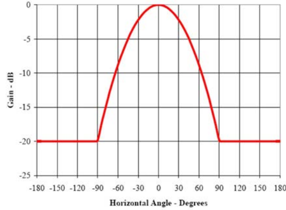
Figure 7.7.4-2 Simplified antenna pattern [ITU-R M.2135].
