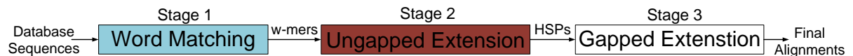
Figure 3.1: Three stages of BLASTN. The first two stages are the bottlenecks. (© 2018 IEEE)
