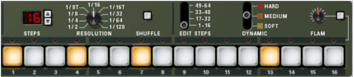
Figure 5.2: Fixed-Grid representation of a 1-measure pattern for a single drum in the interface for Propellerhead’s ReDrum drum machine.
