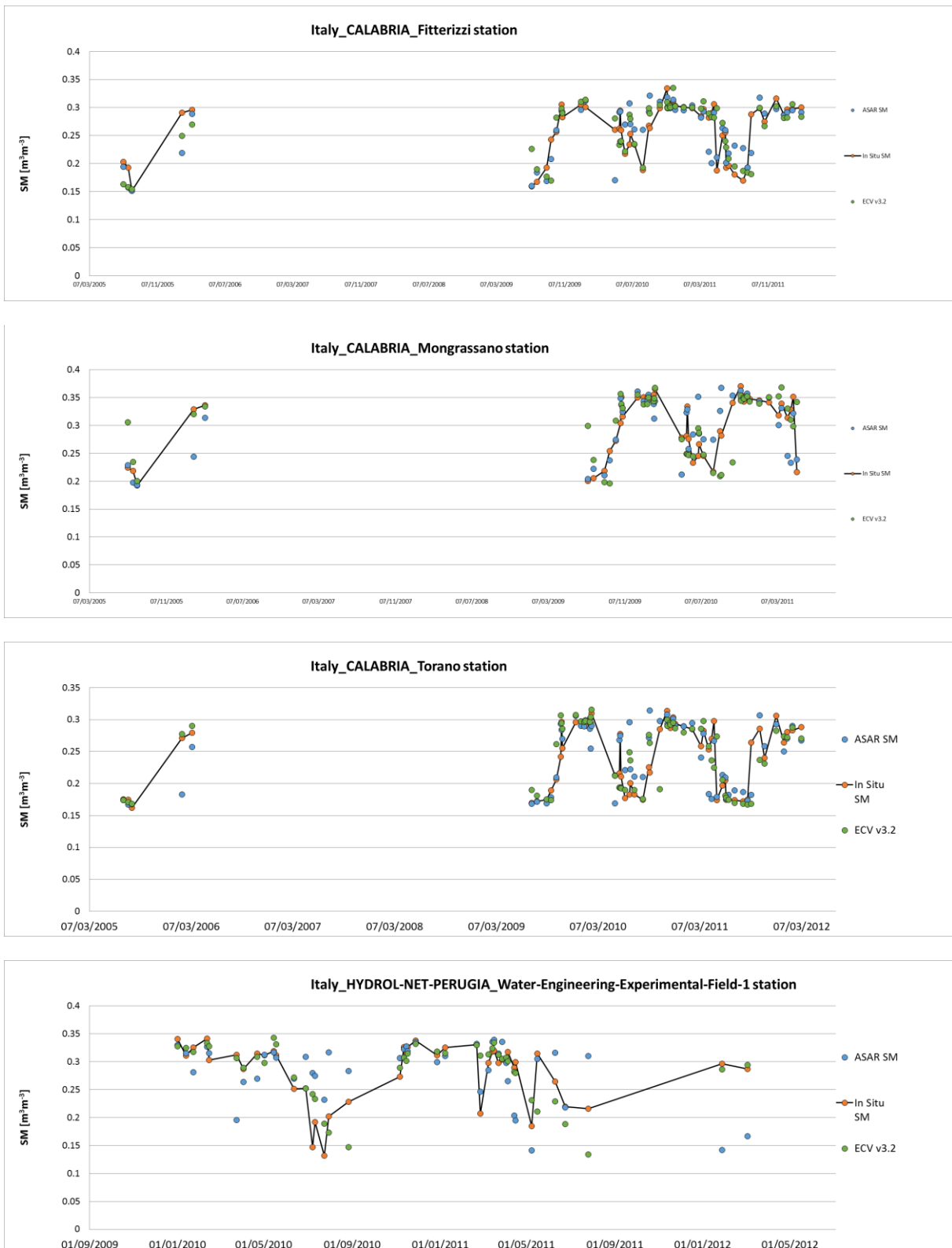
Figure 35: Time series of in-situ, ASAR and ECV SM v03.2 time stations in the Italian regions under investigation. The units are m^3m^{-3} .
