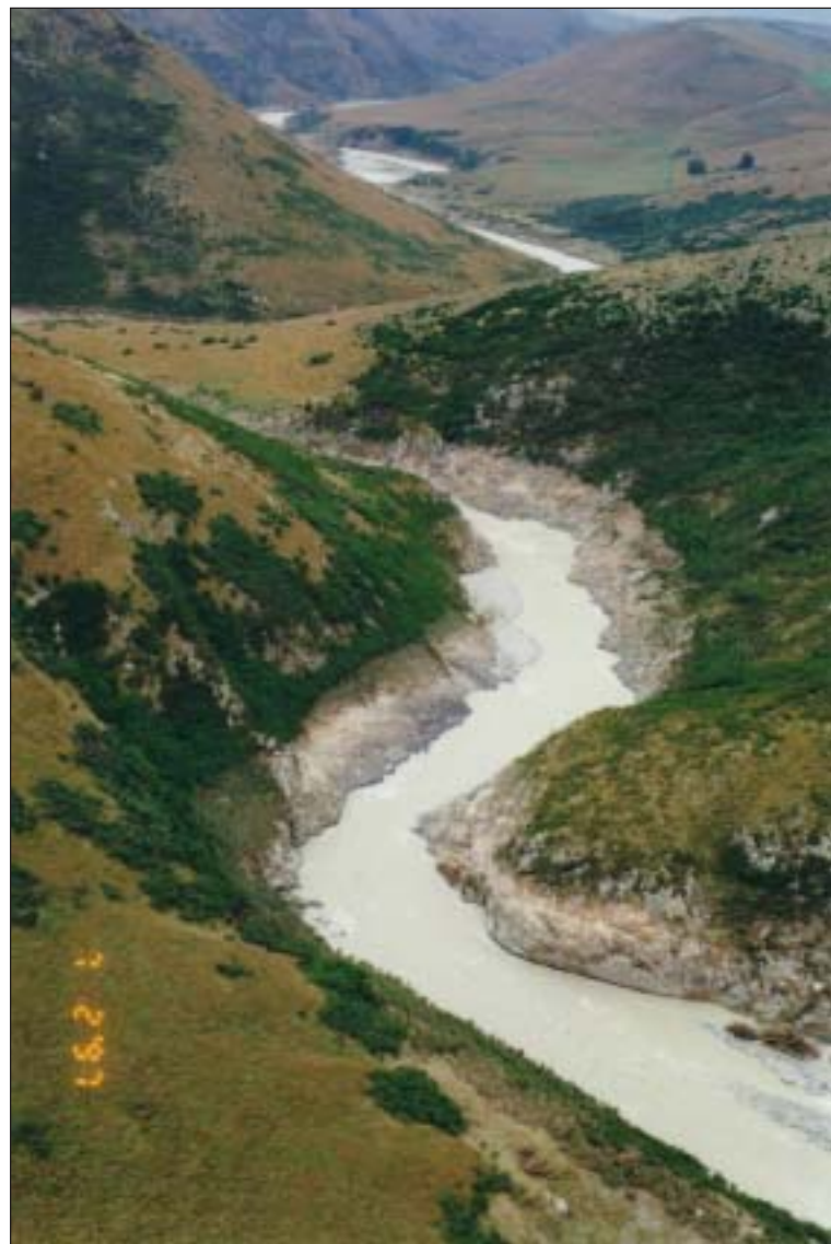
Figure 5. Opuha Gorge, 5 km downstream of Opuha Dam, swept clean of vegetation, soil and water recorders.
