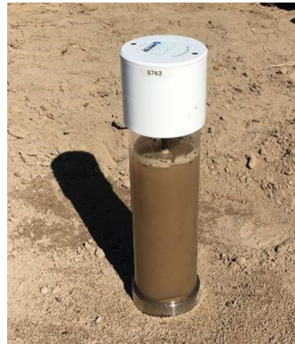
A modified Philip-Dunne infiltrometer, which measures the soil's saturated hydraulic conductivity.
