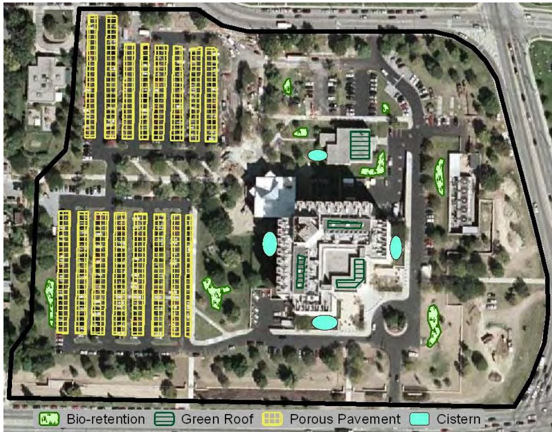
Figure 19. Actual Site and Onsite Control Measures (Cincinnati, OH)
