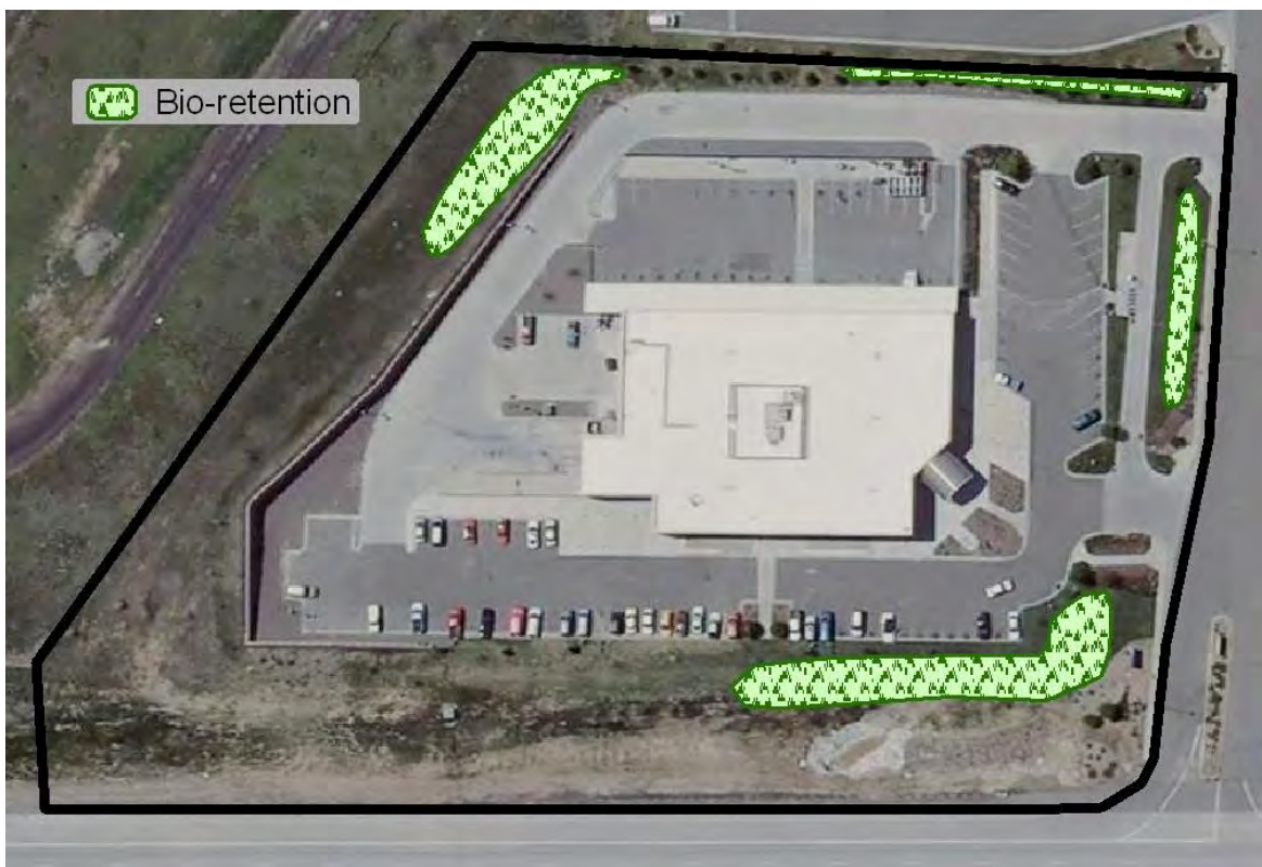
Figure 13. Actual Site and Onsite Control Measures (Denver, CO)
