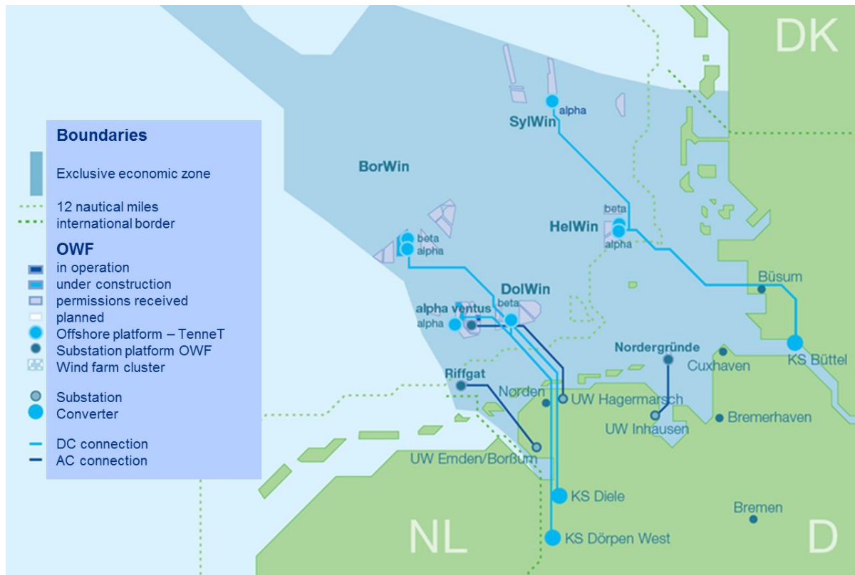
Figure 7.12: Offshore Wind Farms and Grid Connection Systems in the German North Sea
