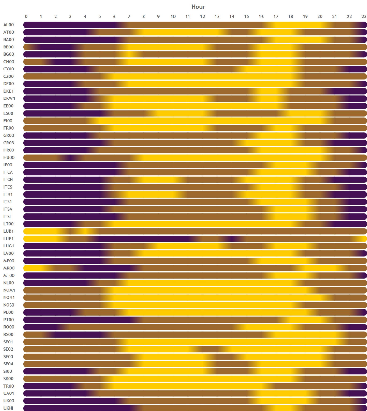
Demand during workdays - mean demand compared with highest mean demand in winter 2021-2022 ■ Less than 75% ■ 75-95% ■ 95-100%
