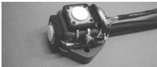
Fig. 4. Polhemus sensor with attached buttons
