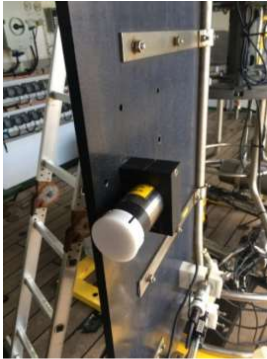
Figure 44. WETLabs BBrted Backscatter Sensor Mounting Location same as DY113 and JC211.
