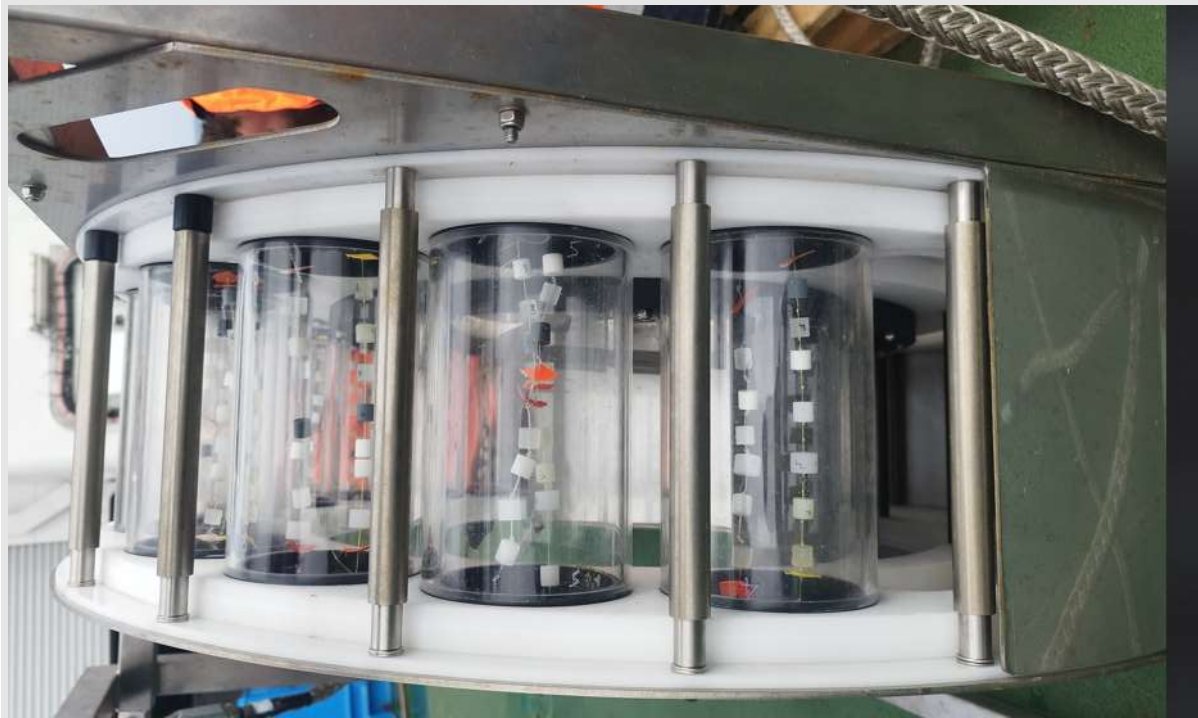
Figure 29. OPIC chambers prepared for deployment. Programming was carried out to move 3 chambers into the ‘garage’ after 8, 12 and 24 months. Chamber 5 was loaded into OPIC upside down therefore the polymer order is transposed.
