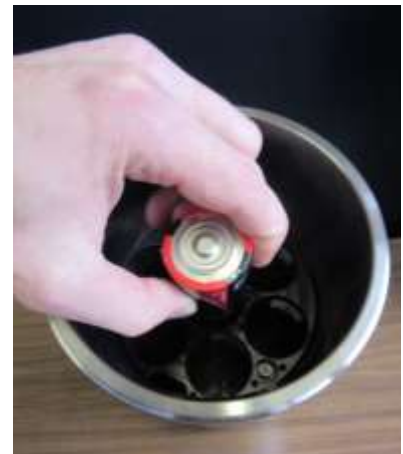
Figure 10. Installing batteries into a battery container.
