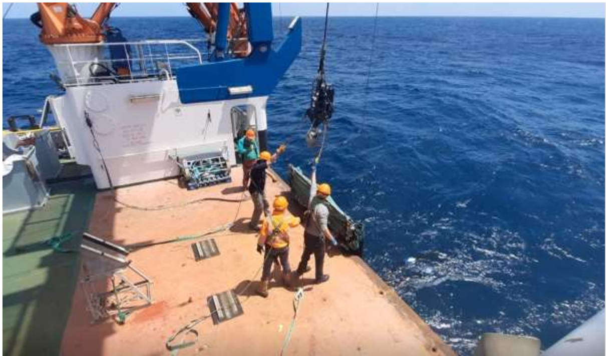
Figure 23. Recovery of RMT8 net. Auxiliary wires connected and weight bar in the process of being hauled on deck by auxiliary winches in tandem with the trawl winch.
