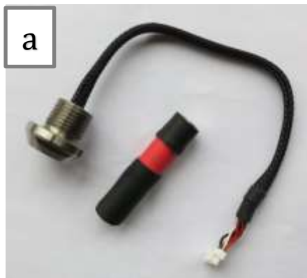
Figure 12. a) Magnet starter plug and included magnet. b) Switching ON the sonovault using the magnet starter plug (black North pole). c) Switching OFF the sonovault using the magnet start plug (red South pole).
