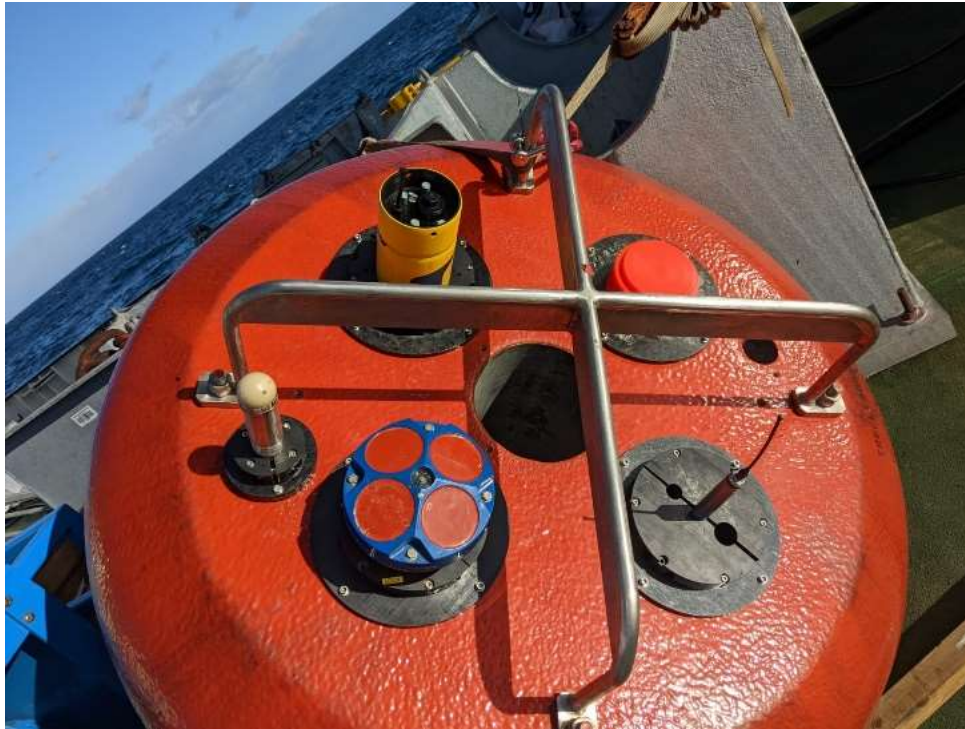
Figure 16. WBAT (top left) and upwards facing 120 kHz transducer (top right) installed into WCB mooring buoy.
