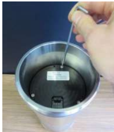
Figure 9. Top view onto battery container.
