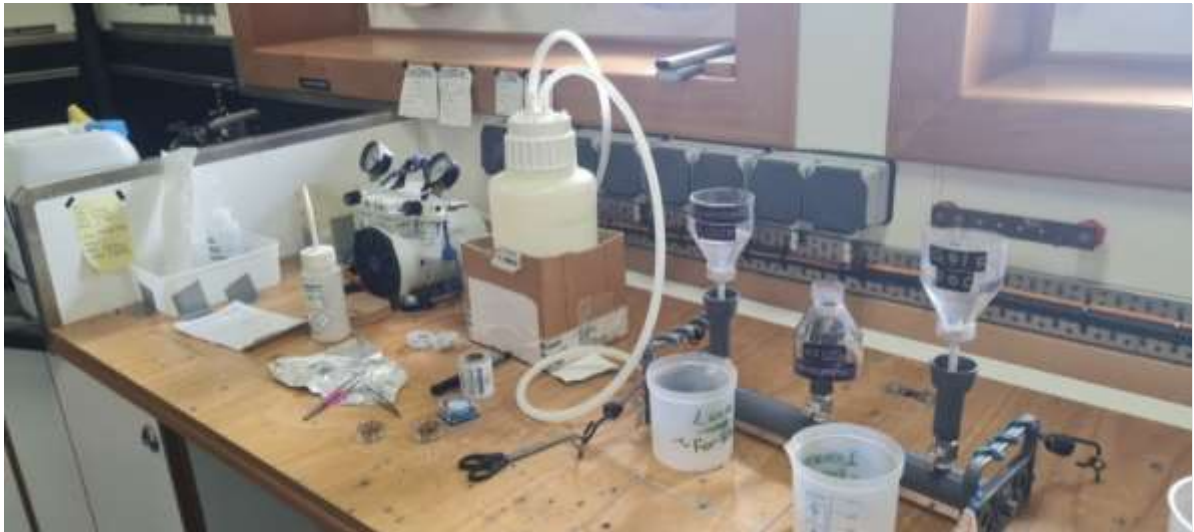
Figure 66. Filtration setup in the general lab.
