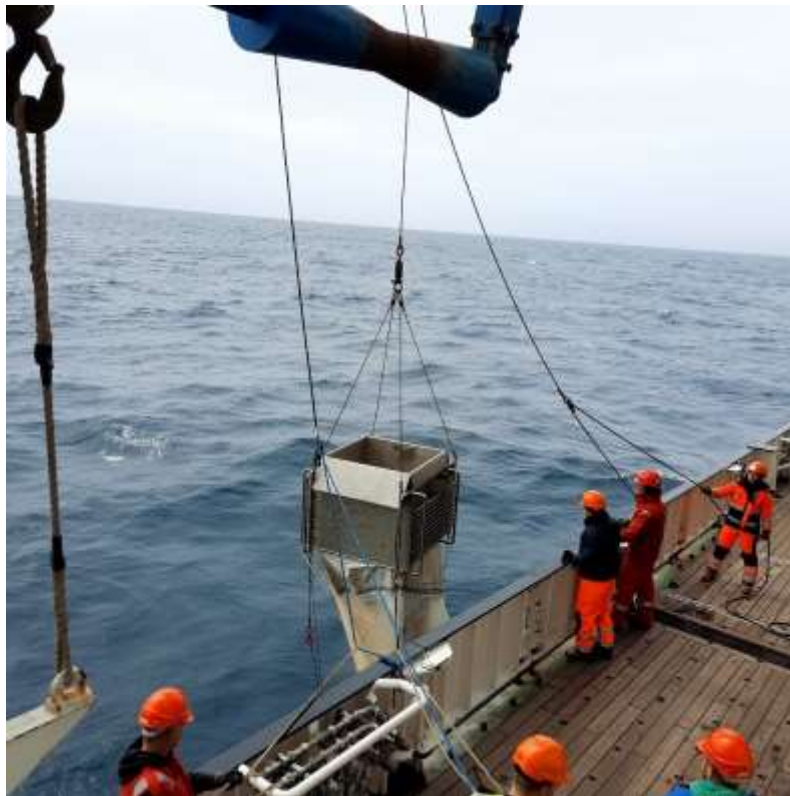
Figure 21. Rexworth winches have now been detached and weight of carousel is now taken by the 4 wires between it and the main body. Retaining ropes (with G links) now hold the carousel deployment wires. Main frame has been rotated 90° sideways to allow an operator to reach and disengage the safety bar before the instrument is lower for deployment.
