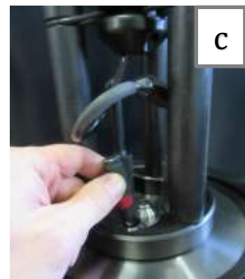
Figure 12. a) Magnet starter plug and included magnet. b) Switching ON the sonovault using the magnet starter plug (black North pole). c) Switching OFF the sonovault using the magnet start plug (red South pole).
