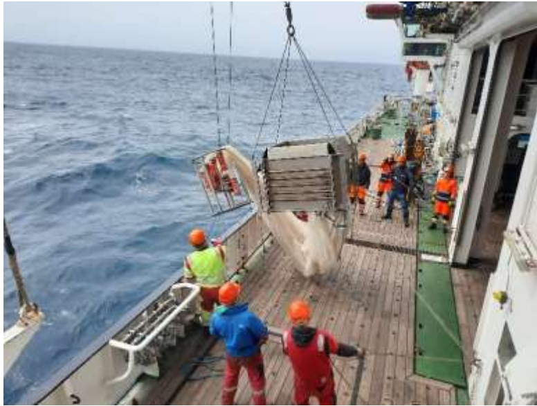
Figure 20. Rexworth winches are used to manoeuvre the cod end carousel outboard while wait of main body is taken by the trawl warp.
