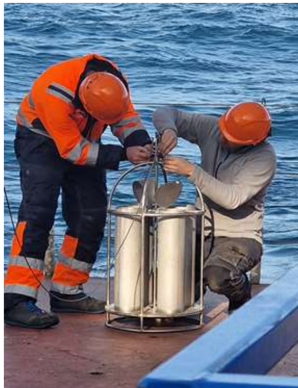
Figure 33. Deployment of floating sediment trap with the detail of the unit including a metal cage and four microplastic collectors. No plastic materials were used to build up the floating trap to avoid contamination; b- schematic of the floating trap deployment.
