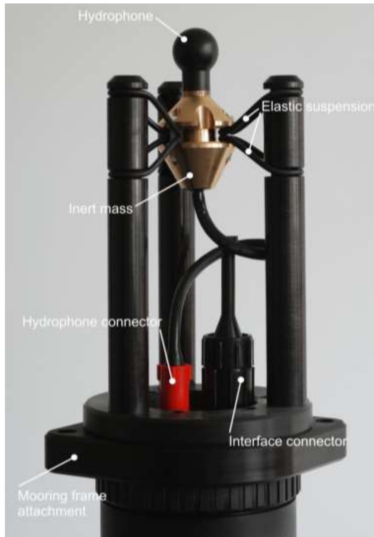
Figure 7. Top section of sonovault, showing hydrophone. Batteries are stored beneath this.
