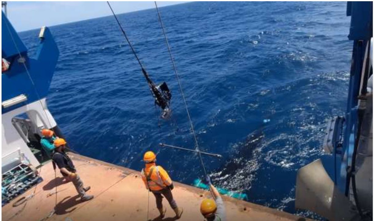
Figure 22. Recovery of RMT 8 net. Auxiliary wires yet to be connected to the weight bridles.
