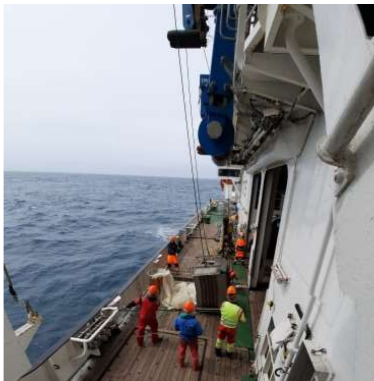
Figure 19. Predeployment – Rexworth winches used to rotate main body so the mouth faces upwards. These winches are then detached and attached to the cod-end carousel for deployment.
