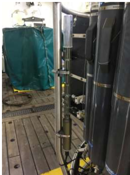
Figure 45. Seabird SBE 35 DOST Mounting Location Overview same as DY113 and JC211.
