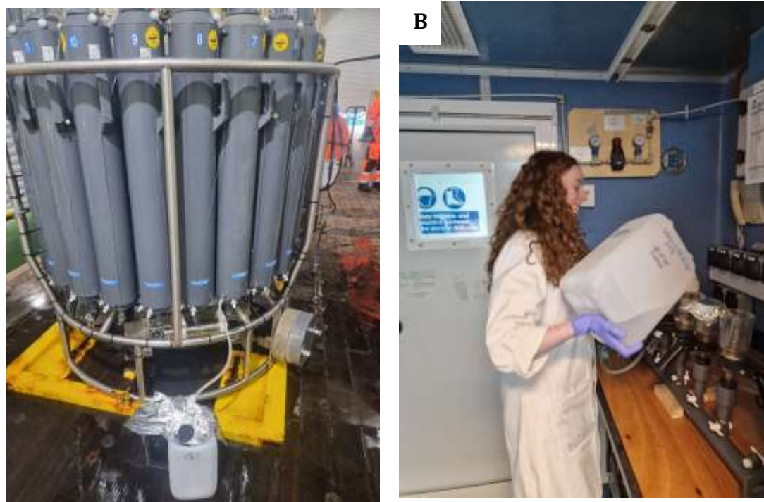
Figure 32. Microplastic sampling from a CTD. A: Filling up of carboy from a Niskin bottle with microplastic contamination precaution in place. B: Filtering MilliQ in preparation for sample processing in the trace metals lab onboard.
