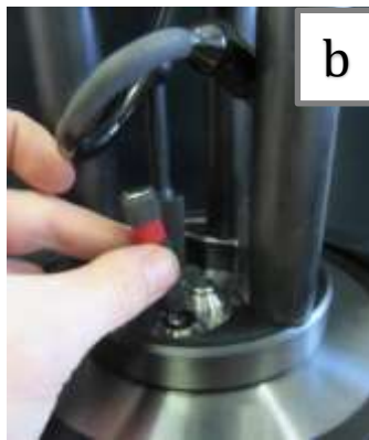
Figure 12. a) Magnet starter plug and included magnet. b) Switching ON the sonovault using the magnet starter plug (black North pole). c) Switching OFF the sonovault using the magnet start plug (red South pole).
