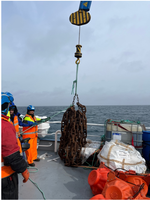
Figure 11. Mooring weight being lifted from bridge deck to port quarter on forecandle deck.
