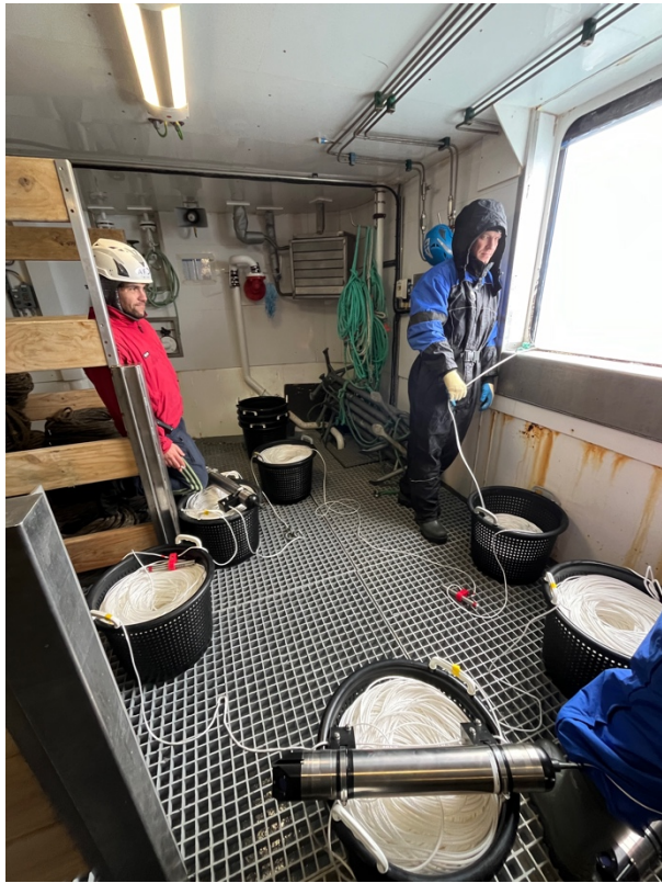
Figure 13. Deploying the mooring rope and instruments through the buoy hatch through the transom in the line magazine room.
