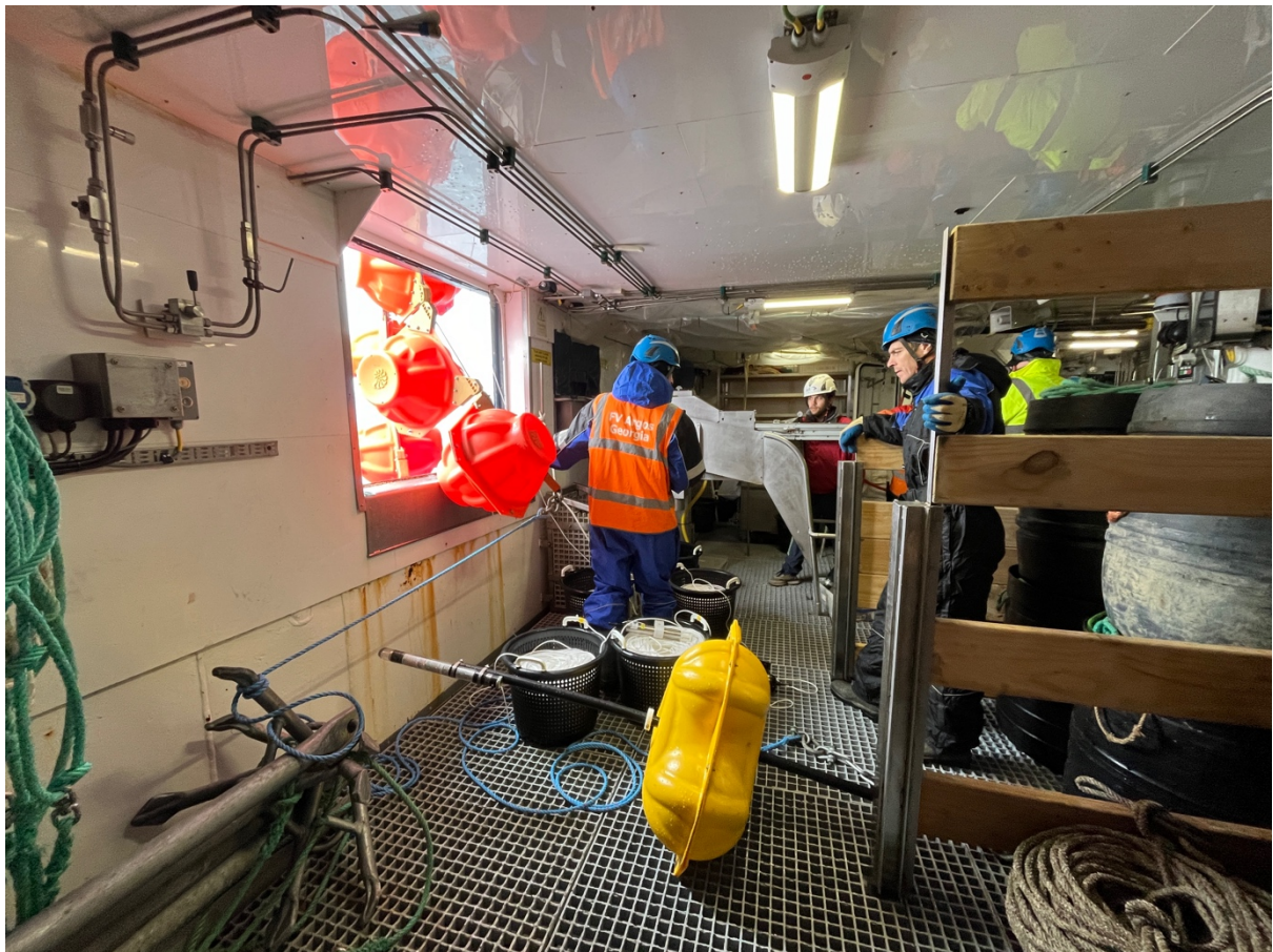
Figure 12. Ends of mooring rope connected to top Eddygrips through the buoy hatch in the line magazine room, ready for deployment.
