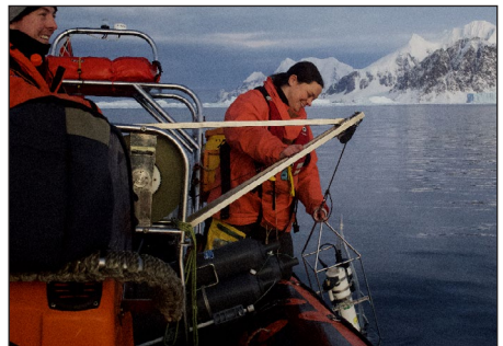
▲ Deploying a CTD on the hand winch to 500m depth
