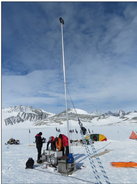
▲ The BAS Rapid Access Isotope Drill (RAID) in action at a previous test site
