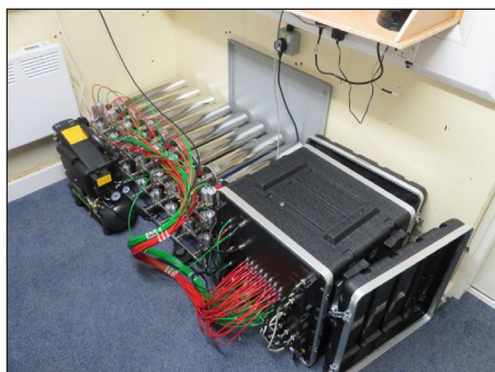
▲ The automated methane flask sampler in the CASLab
