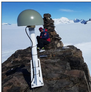
▲ GPS monument and antenna at Traverse Mountains, Antarctic Peninsula
