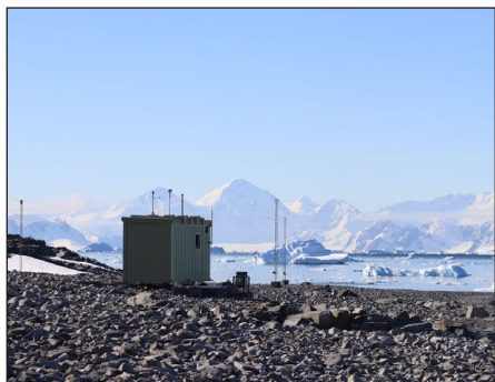
▲ The Rothera Clean Air facility at East Beach was built in the 2021-22 season and will be measuring cloud and aerosol properties for at least four years
