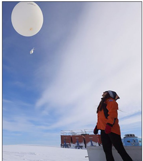
▲ Radiosonde launch at Halley
