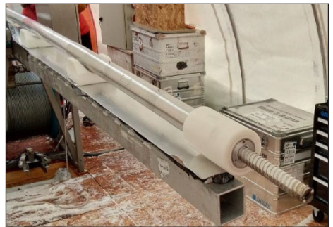
▲ The new P-RAID rock drill with coring barrel extended. We will be testing the P-RAID in conjunction with use of the RAID
