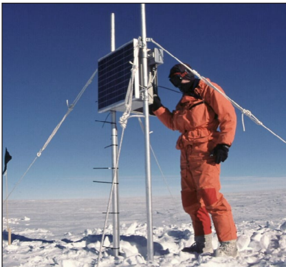
▲ BAS scientist checking the solar power unit for one of the remote Low Power Magnetometers
