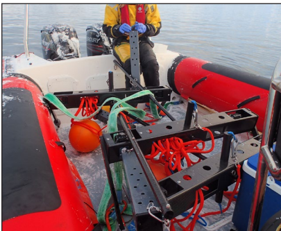
▲ A BRUV (Baited Remote Underwater Video) system being assembled on the boat for deployment
