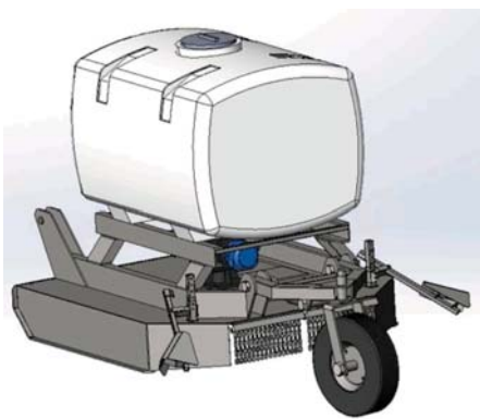
CAD drawings of the combined mower and sprayer for use in Christmas tree cultivation.
