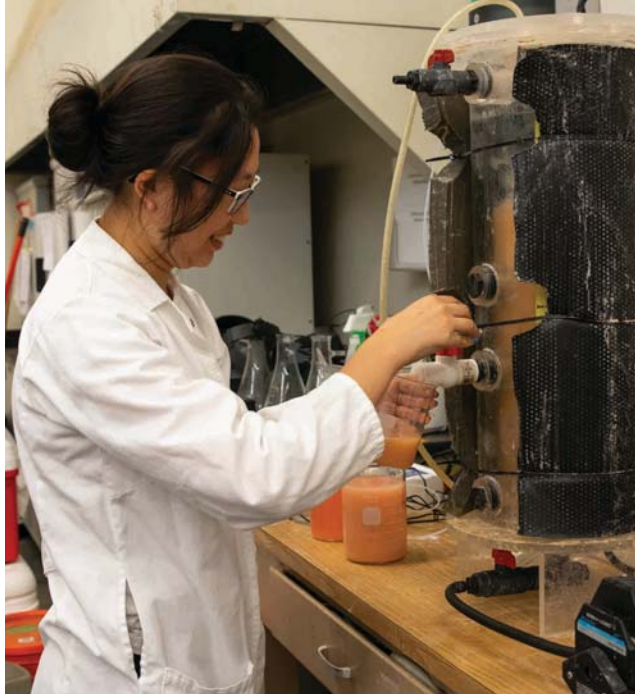
The team takes a liquid sample out of the bioreactor for processing (photo courtesy Katherine Hung/UC Davis).
