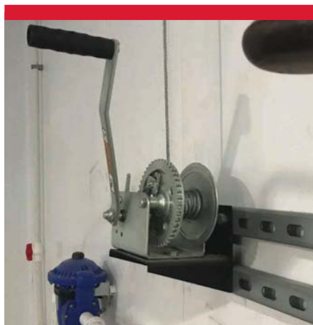
The hand-cranked winch used to raise and lower the feeders.
