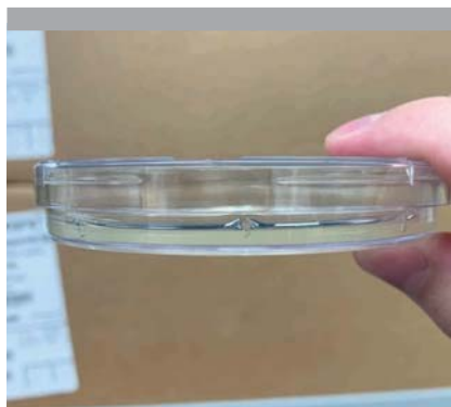
Example of a petri dish with improperly shaped wells. Note the lifted auger in center of the picture.
