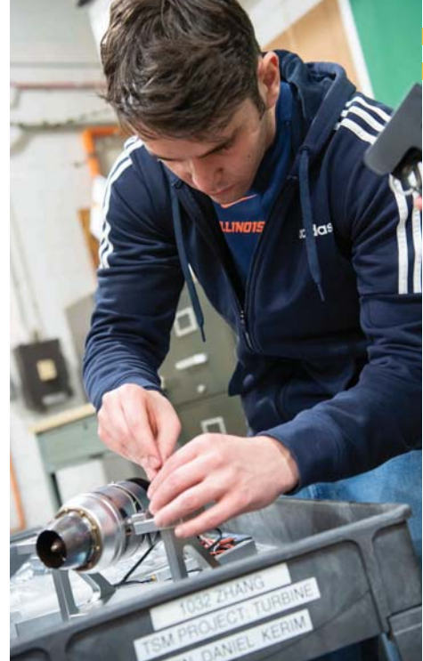
ETMAS Senior Kerim Lakota assembles an RC jet turbine test stand. This test stand will be used to test jet bio-fuels created in the ABE department.
