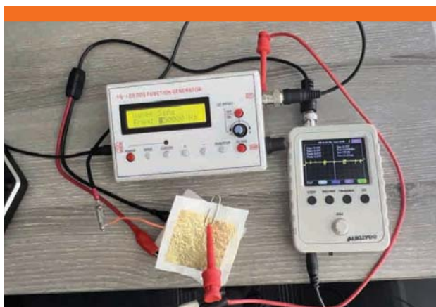
Antenna transmission test with function generator and pocket oscilloscope.
