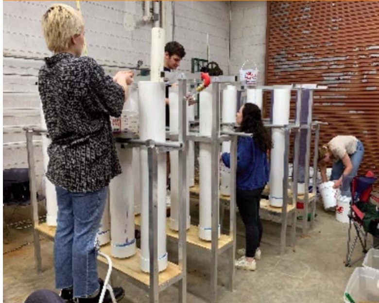
To find a replacement for sand, which has large ecological and carbon footprints, the team developed a column apparatus to test locally sourced waste materials for use as rain garden media. Team members include (left to right) ASABE members Ella Knight, Bryce Miller, Maddie Ginsberg, and Jaimie Armitage.
