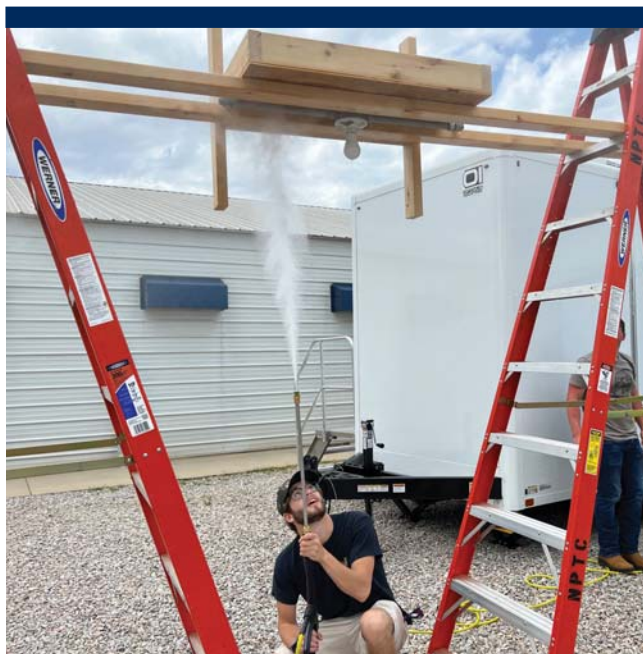
Adam Lenhard performing a water intrusion test that simulates a poultry house washdown.
