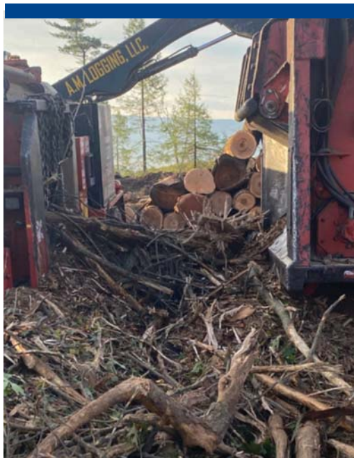
Woody debris from a flail delimeter at A.M. Logging in Centre Hall, Pennsylvania.
