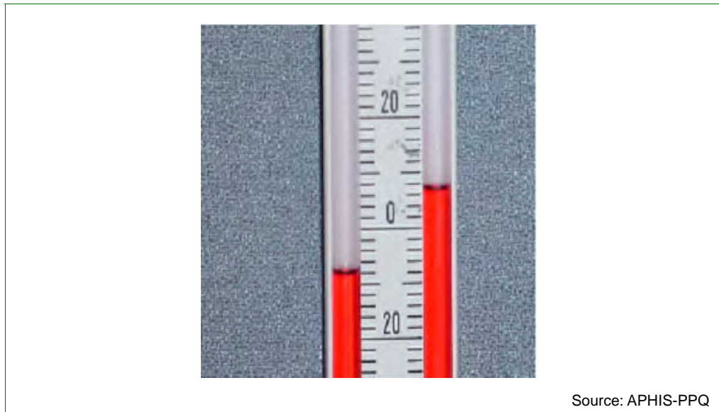
Figure 8-1-8 Example of U Tube Manometer
