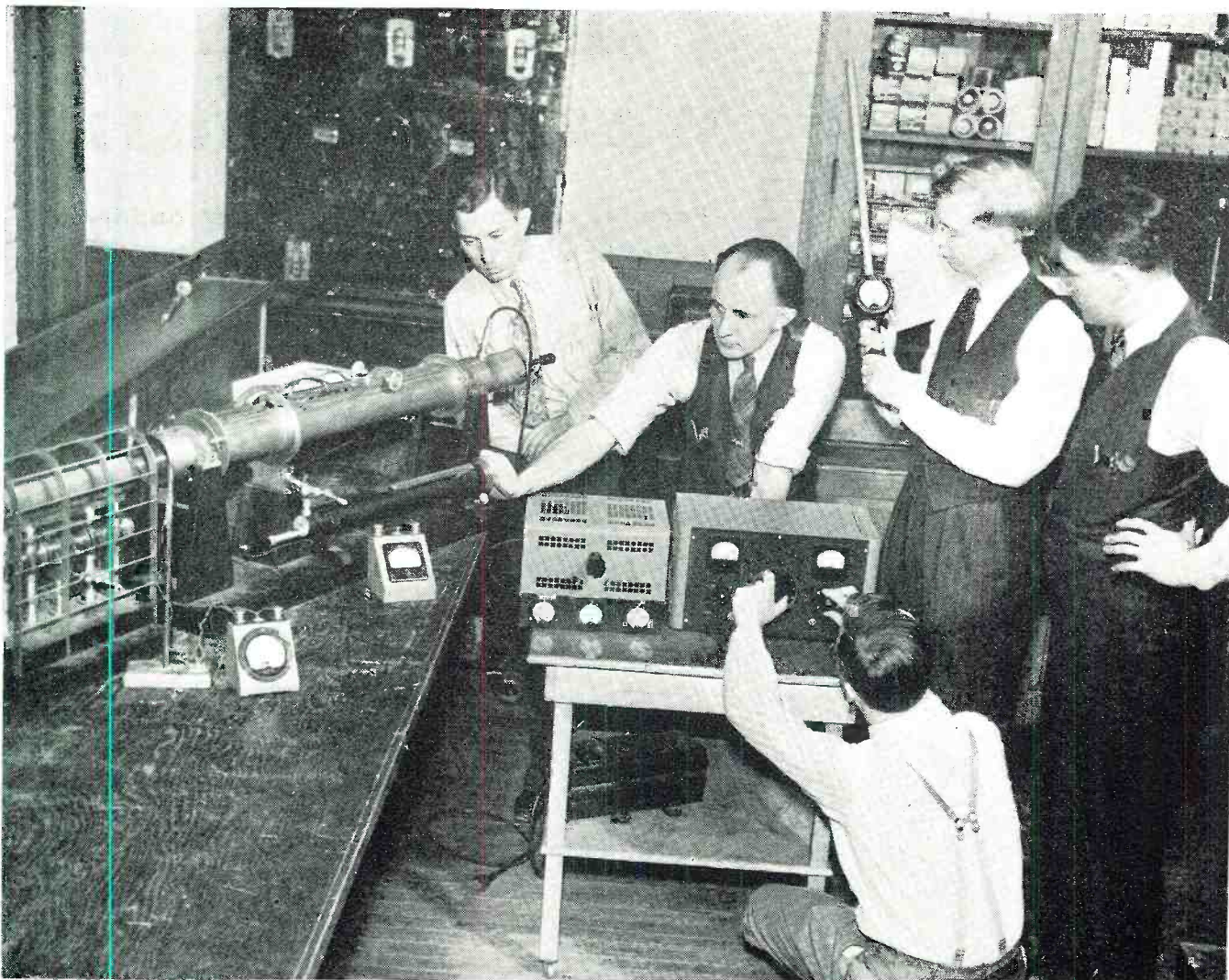
Investigating electromagnetic wave patterns in cylindrical wave guides at 3000 megacycles, using a Klystron oscillator.
