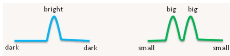
Figure 8 The specific pattern of the numbers of pixels with intensity change when TakePicture Event happens. The left one is the pattern in normal frame, and the right one is the pattern in frame differencing
