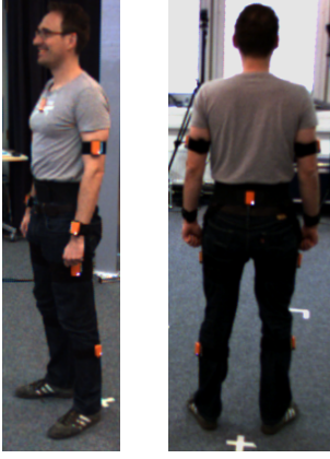
Fig. 7: Sensor placement: 10 sensors are strapped to body extremities (shank, thigh, forearm, upper arm), chest and waist.
