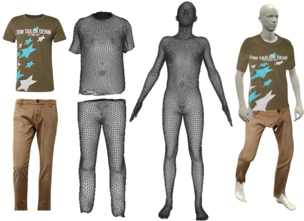
Figure 2. Given regular online retail store images, our method can automatically produce textures for pre-defined garment templates, that can be used to virtually dress SMPL [42] in 3D.
