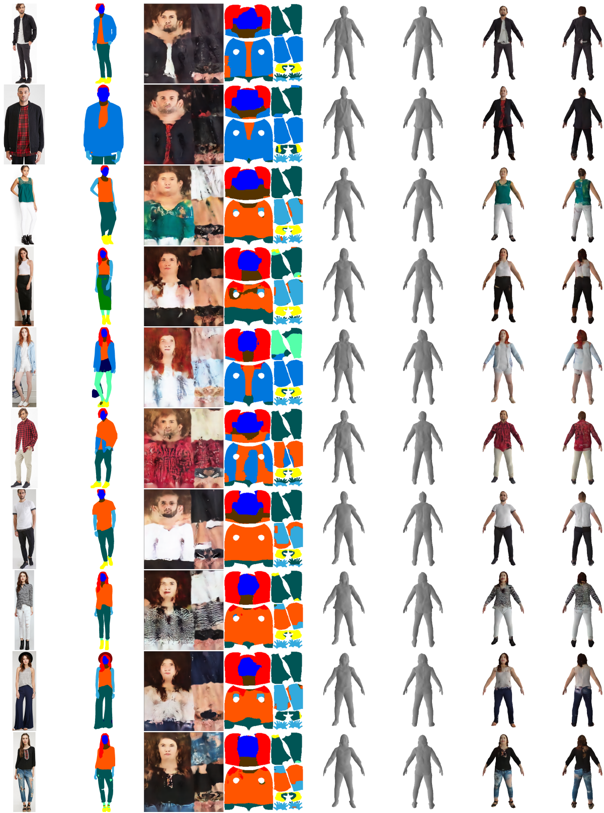
Figure 5: Image to 3D model, randomly selected results. Left to right: real image, segmented image, complete texture map, complete segmentation map, generated untextured avatar, generated textured avatar.
