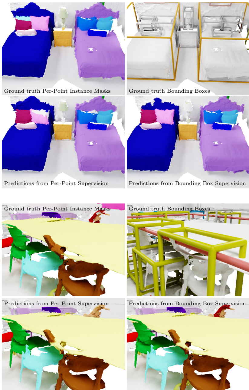
Fig. 12: Qualitative Instance Segmentation Results on ScanNet [9] Individual instance masks are colored randomly and match the ground truth instance mask colors. Left: results from full per-point supervision. Right: weak bounding-box supervision.
