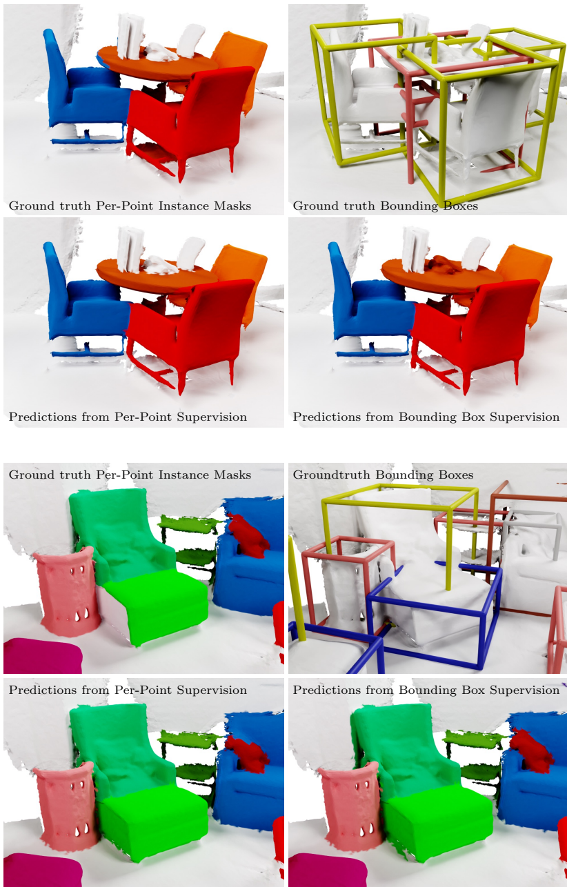
Fig. 11: Qualitative Instance Segmentation Results on ScanNet [9] Individual instance masks are colored randomly and match the ground truth instance mask colors. Left: results from full per-point supervision. Right: weak bounding-box supervision.
