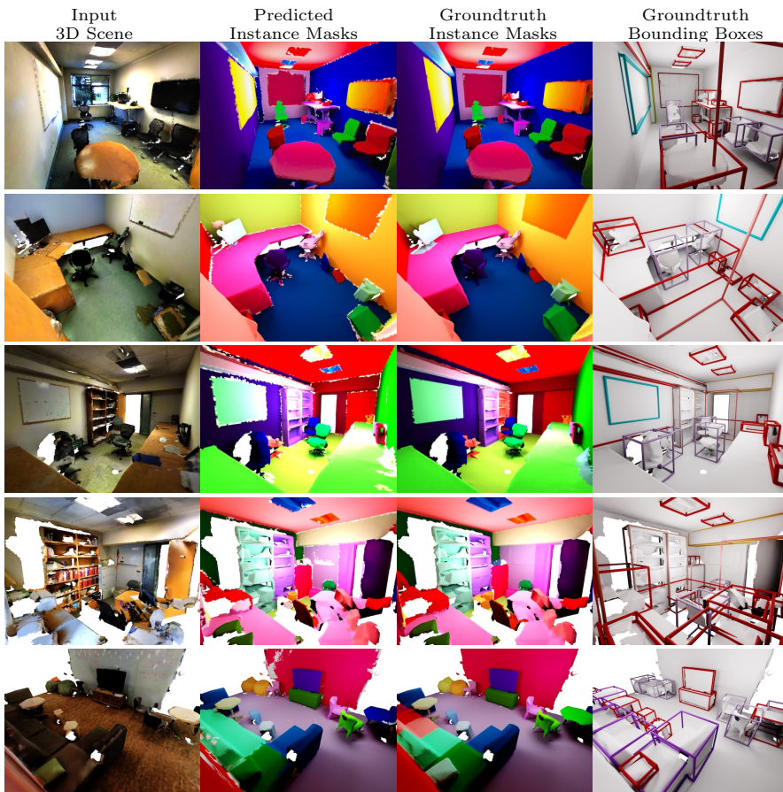
Fig. 10: Qualitative Instance Segmentation Results on S3DIS [2] Individual instance masks are colored randomly and match the ground truth instance mask colors. During training, only bounding box annotations are used (last column), per-point instance masks (third column) are not used, and are shown here only for judging the quality of the predicted instance masks (second column).
