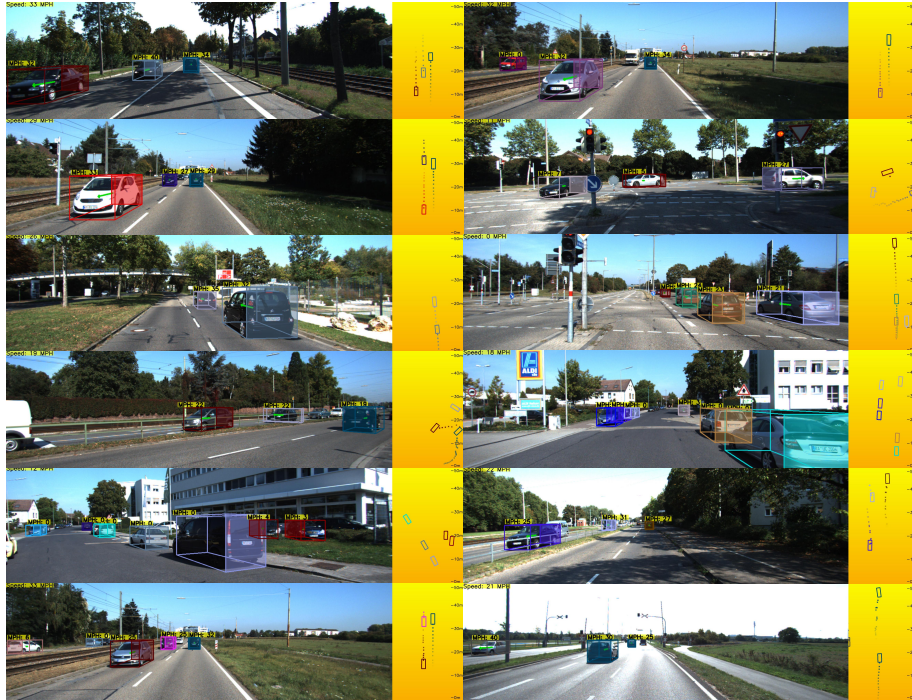
Fig. 6. Qualitative Examples. We depict the image view (left) and BEV (right). We show velocity vector in green, speed and ego-motion in miles per hour (MPH) on top of detection boxes and at the top-left corner, and tracks as dots in BEV.
