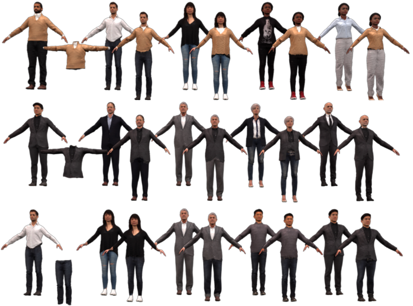
Figure 4: Texture transfer. We model each garment class as a mesh with fixed topology and surface parametrization. This enables us to transfer texture from any garment to any other registered instance of the same class. Rows correspond to shirt, coat and pant respectively. The first column shows the source garment mesh, while the subsequent images show original and transferred garment texture registrations.
