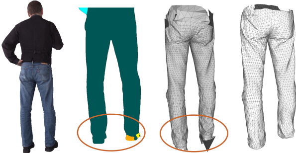
Figure 2: Robust segmentation is essential to register garments without artifacts. Here we can clearly see that incorrect segmentation leads to artifacts in registration. From left to right: scan, erroneous segmentation of feet, distorted pant registration, registration with corrected segmentation.
