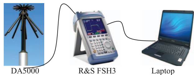
Figure 1. Measurement equipment configuration.
