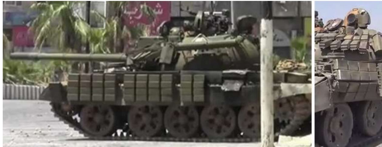
Explosive reactive armor (ERA) applique to tank front glacis, turret, and sides
