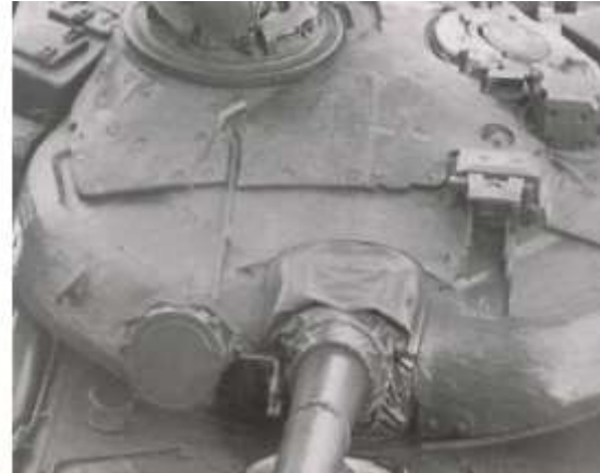
"Bra"-type armor applique on turret front-plates on top
