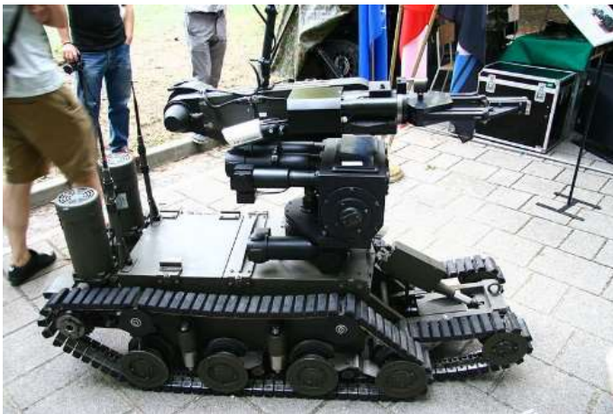
Figure 1: Inspector Mid-Sized Robot, Poland
