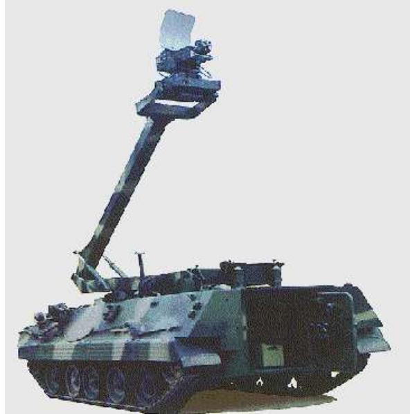
HJ-62C with Mast in Raised Position
