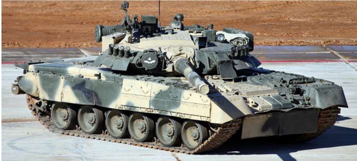
“Clamshell-type” turret armor applique and skirts, front applique armor, turret top plates, and side armor skirts
