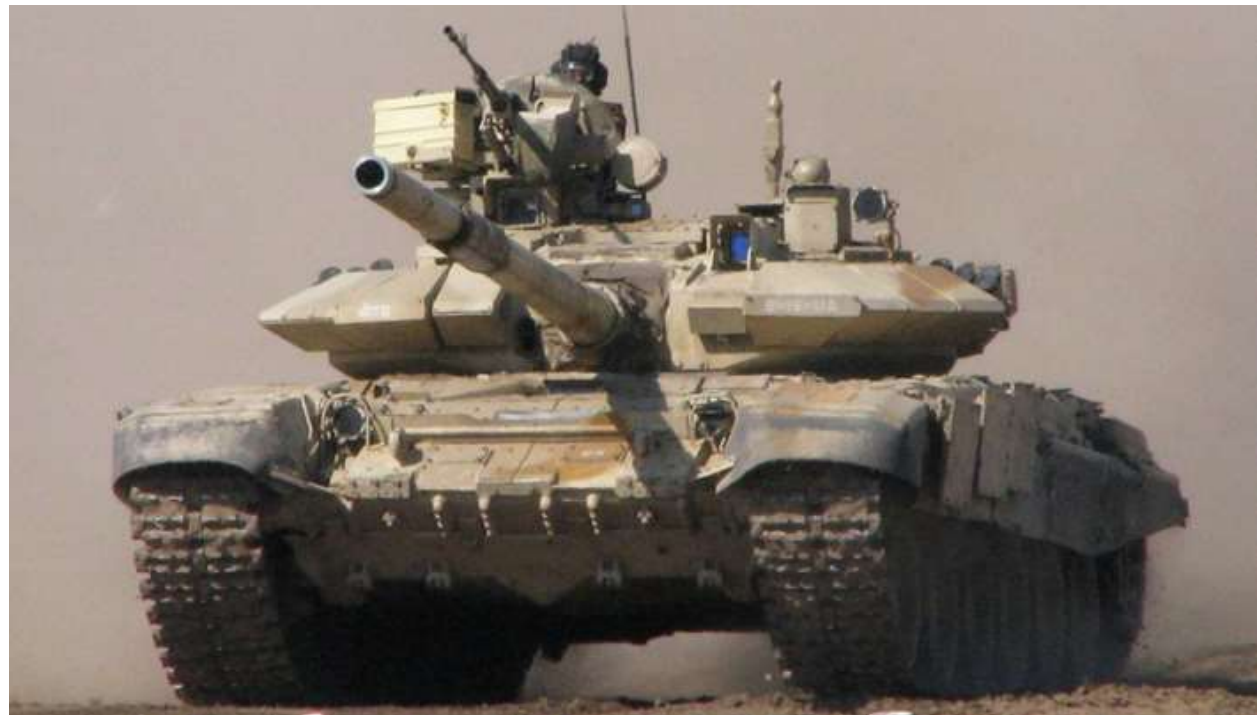
"Clamshell-type" armor applique, front applique armor, turret top and side skirt armor plates
