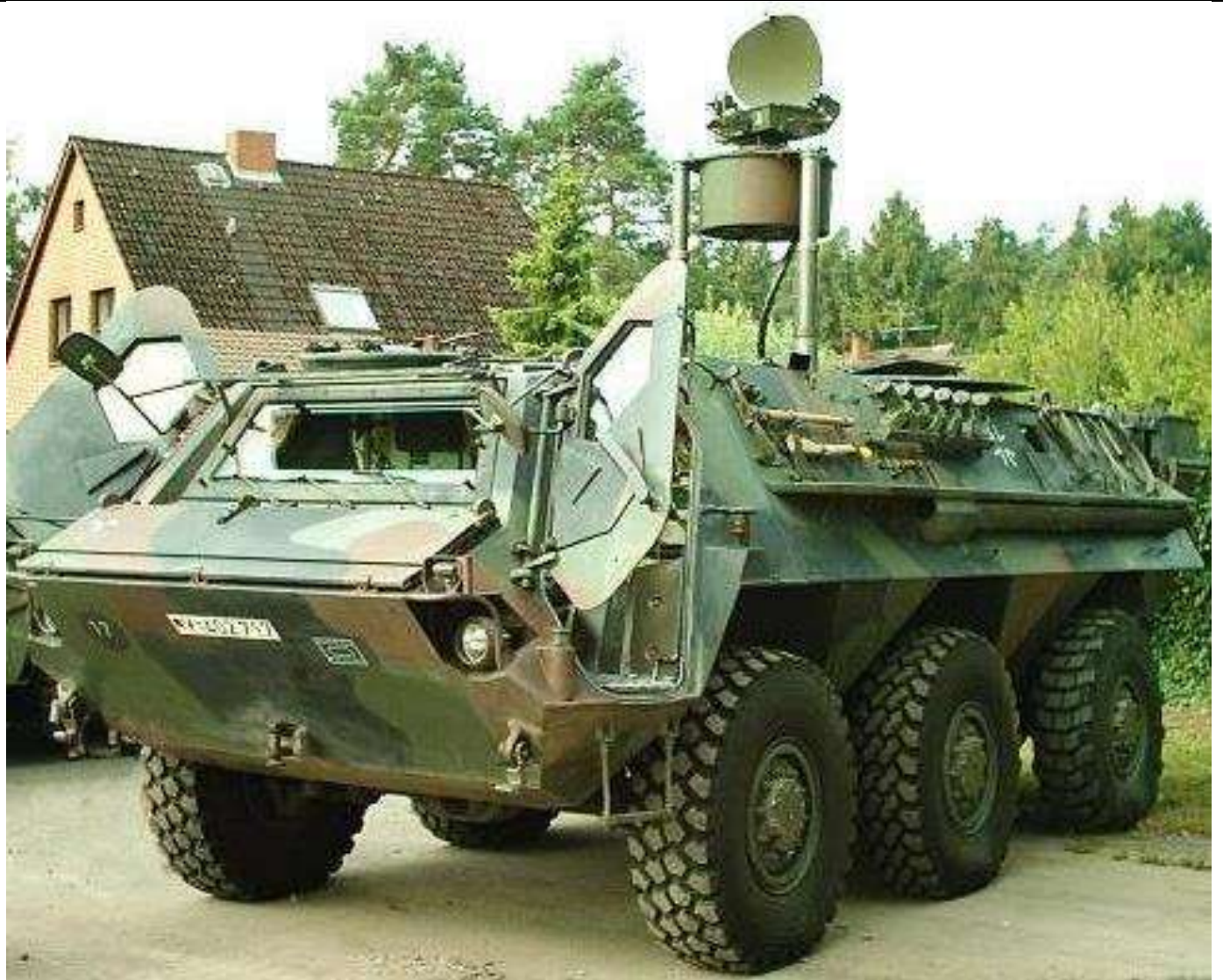
RASIT Ground Surveillance Radar (GSR) Mounted on Vehicle
