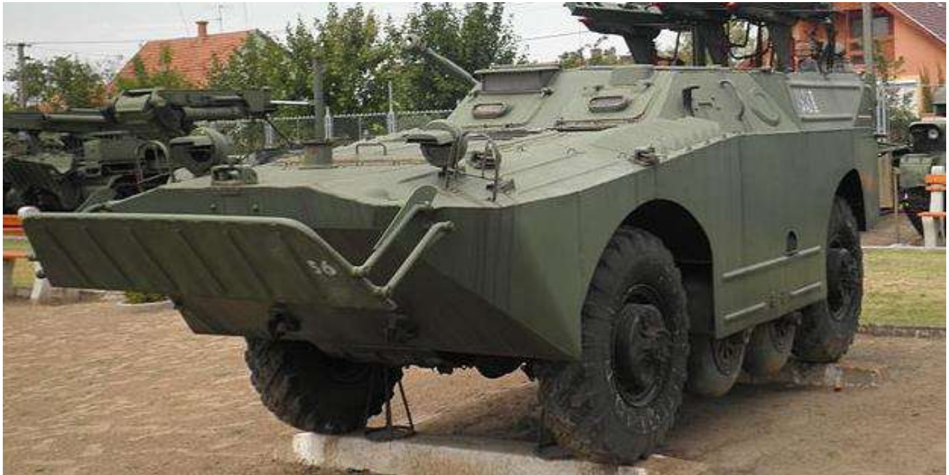
BRDM-1 converted to an ATGM platform
