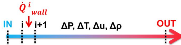
Figure 3. Sketch representing the coolant evolution through the cooling circuit.
