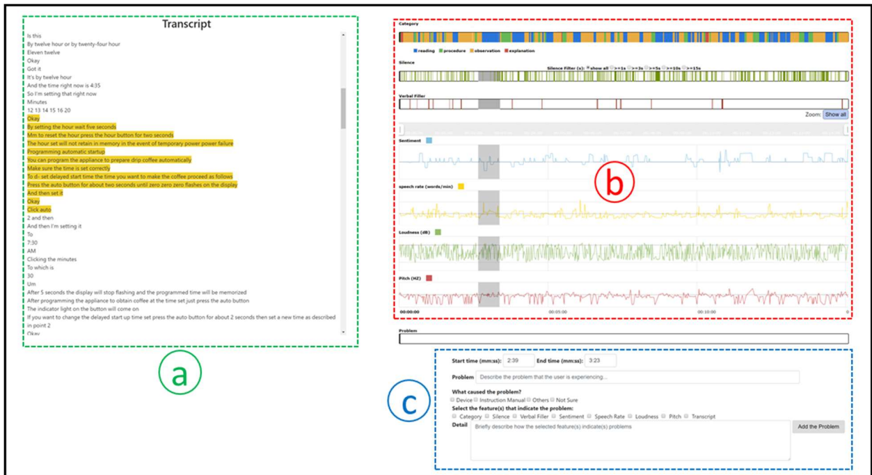
Figure 25. The updated tool for evaluators to analyze recorded think-aloud sessions. It visualizes the transcript of the recording on the left panel (a), one line per audio segment. The seven features (i.e., category, silence, verbal fillers, sentiment, speech rate, loudness, pitch) are represented as time-synchronized charts on the right panel (b). Selecting any part of a chart highlights the corresponding transcript on the left panel. The bottom of the tool (c) allows for describing usability problems and the features used to identify the problems.
