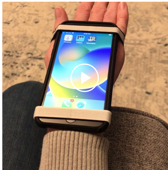
Video 1 Application Demonstration. Demonstration of user beginning a treatment session with the Tremor Retrainer application, including initial measurement of baseline oscillatory movement and biofeedback to reflect the user's accuracy in reaching goal frequency of voluntary movement. After stopping a session, the user can view a log of duration completed.
