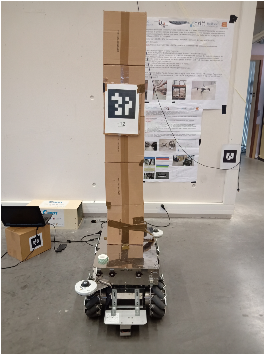
Figure C.2: Summit XL Steel omni ground mobile robot with a tower augmented with fiducial marker.
