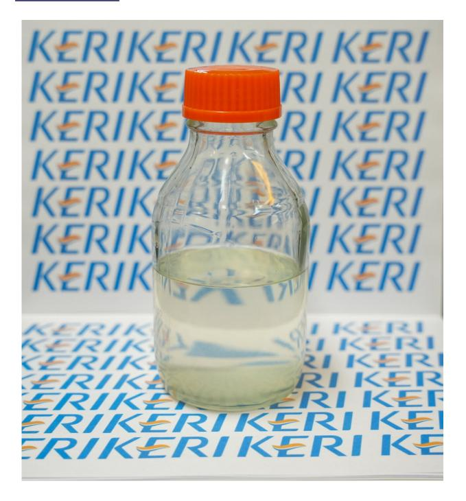
KERI has developed a battery positive electrode binder that can replace PVDF using siloxane. Credit: Korea Electrotechnology Research Institute
