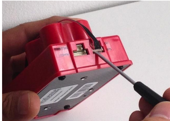
Figure 17: Removal of Connectors Using Small Flathead Screwdriver
