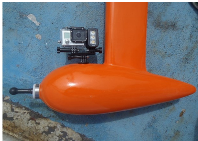
Figure 6 Hydrophone, camera and LED lighting attached to the Hydropod.
