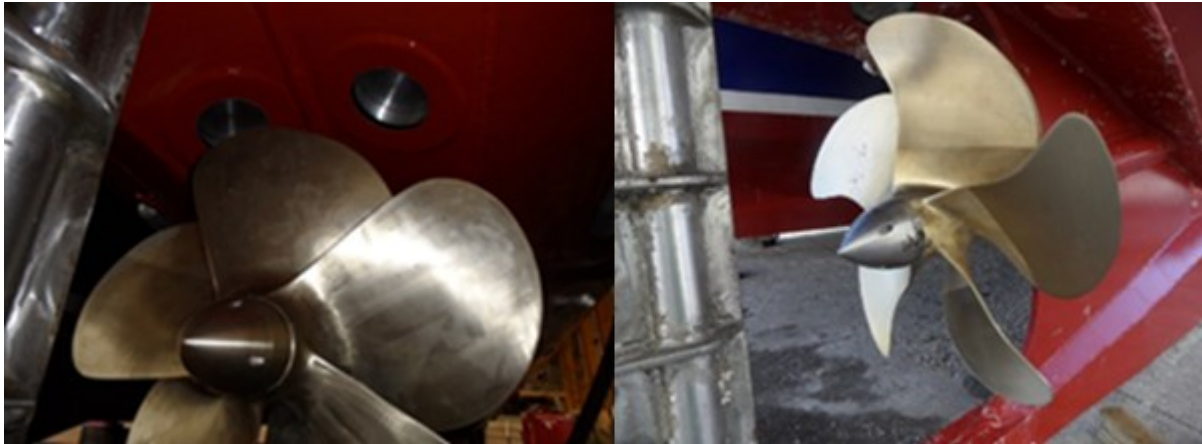
Figure 4 Conventional (Left) and NPT (Right) propeller of “The Princess Royal”
