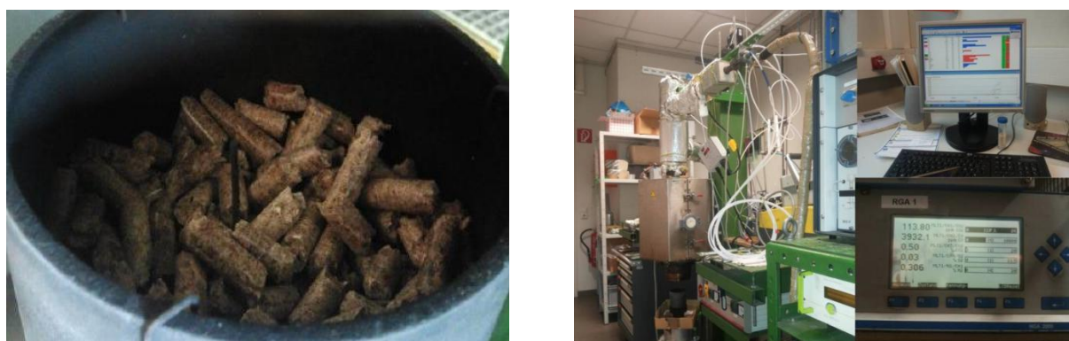
50 Fig. 1. Sample holder with Biomass inserted in the reactor (left); Labr eactor setup (right)
