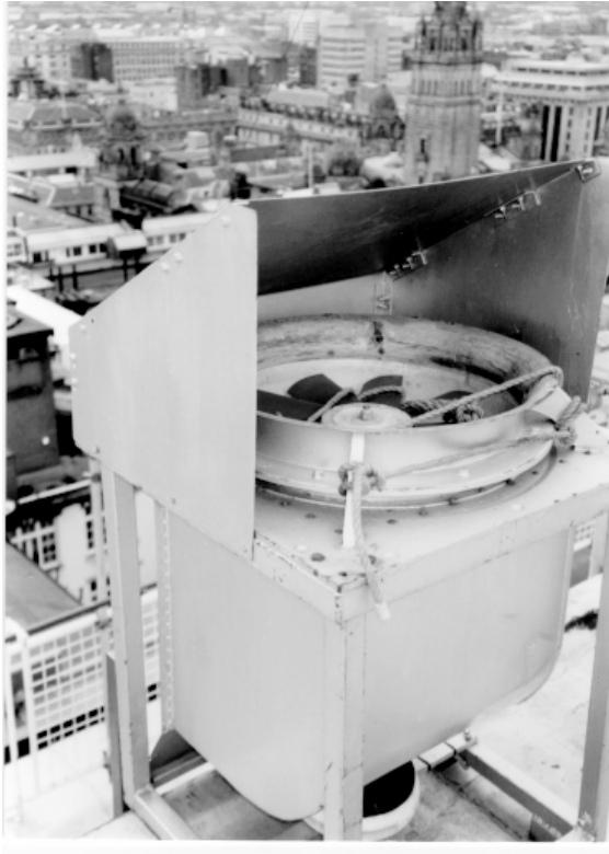
Figure 2: Early ducted turbine prototype under test at University of Strathclyde, Glasgow
