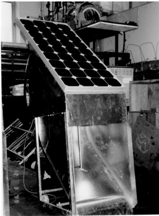
Figure 2: Early ducted turbine prototype under test at University of Strathclyde, Glasgow
