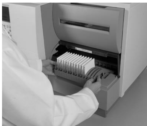
Figure 4. VITEK 2 Cassette Loaded with Cards and Suspension Tubes Being Loaded Into the Automatic Transport System.
