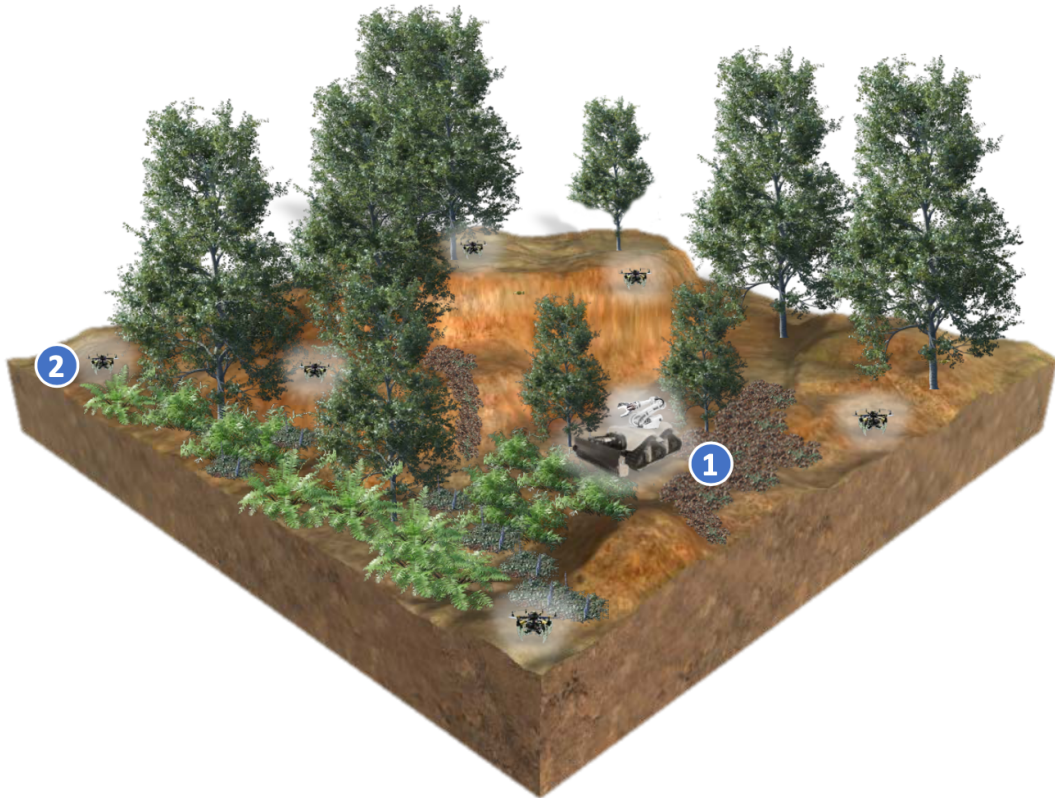
Figure 1: Illustration of the heterogeneous multi-robot system deployment in the SEMFIRE project: 1) the Ranger, a large-sized powerful tracked mobile mulcher; 2) a Scout a small assistive flying robot and member of a fleet of such robots, that can help in exploring and supervising wide forestry areas and aid in the Ranger's navigation capabilities. Figure reproduced from [16].
